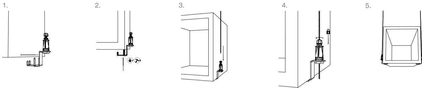
Maximum off axis suspension = 15° (unless otherwise specified by Gripple Technical Services)
